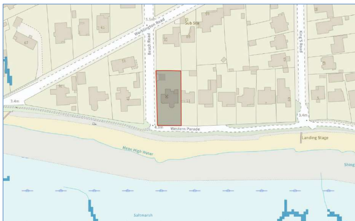
Figure 3 - extract from the EA's Risk of Flooding Surface Water (RoFSW) for the 0.1% AEP
