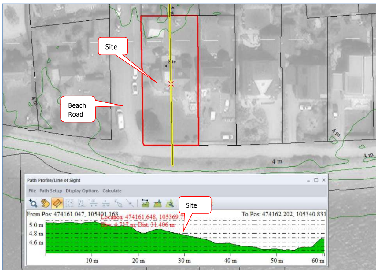
Figure 4 –Terrain profile and contours (source: DEFRA Lidar Data 1m)
