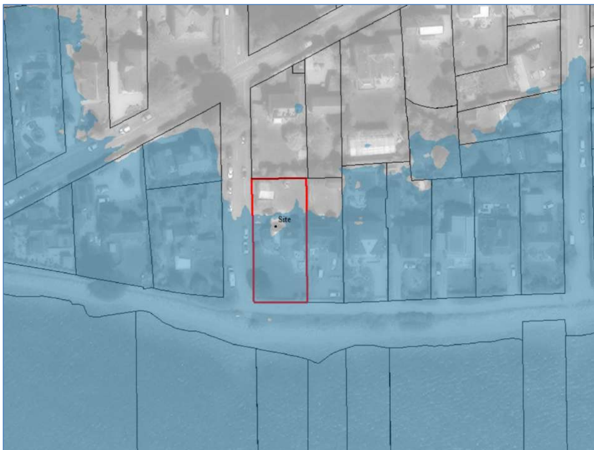
Figure 8 – showing the DFE based on the DFL of 4.849m AOD.
