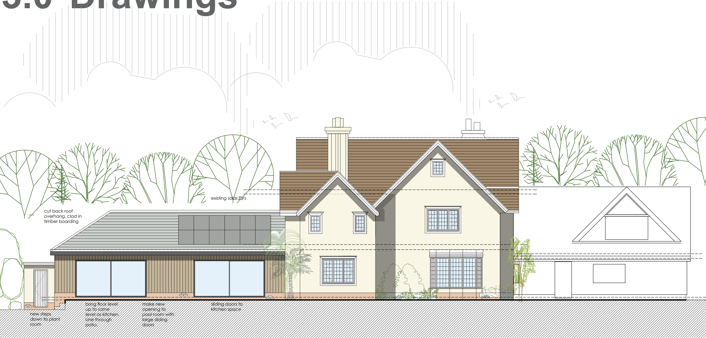
04 Proposed side elevation (pool side) 1:100
