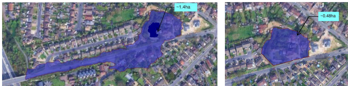
Figure 3 – Estimated Environment Agency catchment (left) vs catchment with local controls applied (right)
