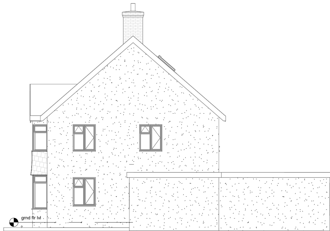
Existing Elevation-Right side
