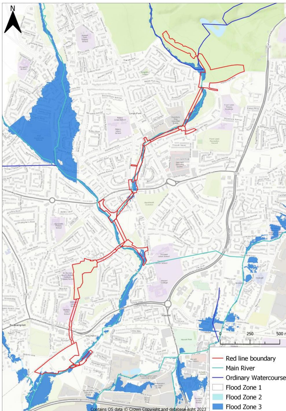
Figure 3.3 - Flood zones across the pipeline route
